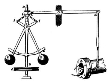
Fig. 1 The centrifugal governor for the steam engine designed by Watt. See text for details
